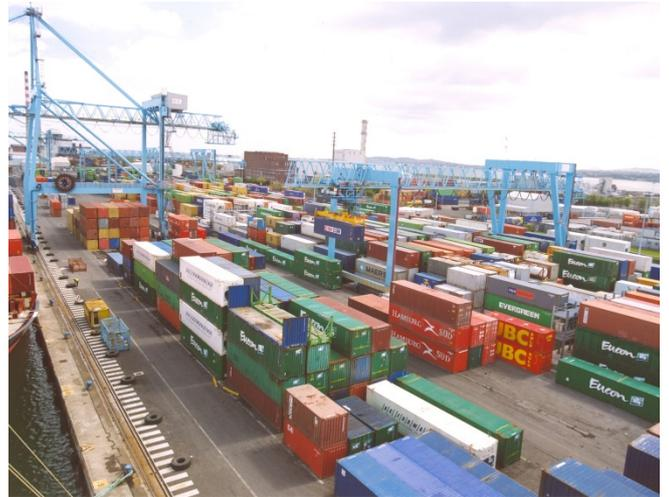
Containers are moved between the stacks and the quay side cranes by special heavy duty truck and trailer combinations or by reach stackers.
